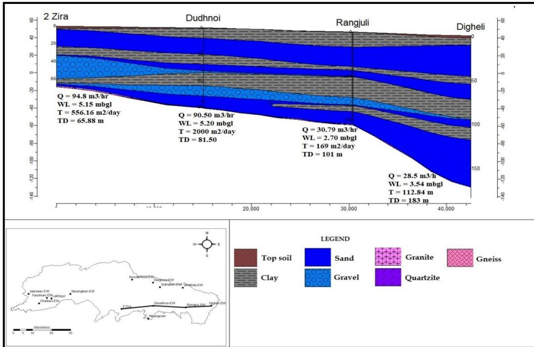
Figure 3.1. 2D disposition along East-West direction.
